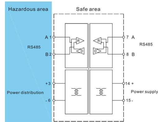
○ The transmission cable in the figure is recommended to use the shielded twisted pair.
