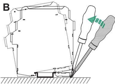
B. Pry the metal lock off the rail with screwdriver as arrow
