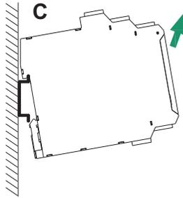
C. Remove the safety barrier as arrow shows.
