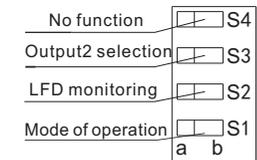
The position of DIP switch has been preset correctly before delivery, please do not change it without necessary.
