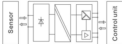
The apparatus can convert the dry contact or NAMUR signals into delay signals, it reflects the apparatus status by the LED indicators on the front side.
